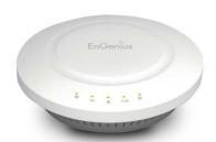
EAP900H equips with two powerful independent RF interfaces that support 2.4GHz 802.11b/g/n (3T3R) and 5GHz 802.11a/n (3T3R), offering bandwidth up to 450Mbps + 450Mbps to accommodate traffic-intensive applications such as multimedia streaming.
